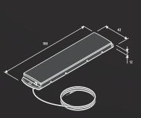
Rotation through 180° allows the alignment of the photocells irrespective of the way they are fixed to the base
